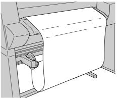
**13** Install the weight roll (a) and weight joint (b) according to the width of the roll media.
